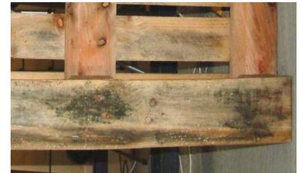
Where timber full-perimeter pallets are in common storage mode in piles laying flat, a third of boards in the pile are tightly compressed by the baseboard of the pallet above. Drying air has no access and these 'tight joints' can remain moist for weeks. That is a perfect breeding condition for sapstain (also known as blue stain) shown lower picture.
