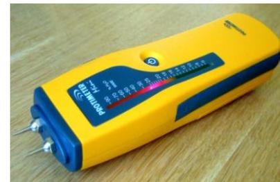
**Fig 1:** Protimeter *resistance type* pocket size moisture meter
